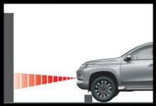
Reduces accidents resulting from abruptly pressing the accelerator from standstill position by detecting obstacles in front or behind the New Montero Sport. (GT 4WD)
