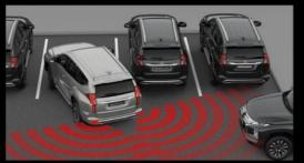
The driver is alerted when the rear radar sensors detect approaching vehicles nearby while the reverse gear is engaged. A warning message appears in the multi-information display, a buzzer sounds, and an indicator blinks in both side view mirrors. (GT 4WD)
