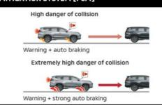
When there is a risk of collision, the FCM system alerts the driver with a visual and audible warning. If the driver does not respond, the system automatically applies moderate to emergency braking. (GT 4WD)
