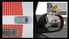
BSW together with the LCA helps the driver avoid sideswiping another vehicle when changing lanes by detecting vehicles at its rear quarters and alerting the driver with an audible alert and a flashing light in the side view mirror. (GT 4WD)
