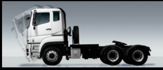
Simplified Serviceability Tilting cab provides easy access to engine bay
