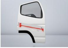
The high-performance suspension Side impact beams built into the doors strengthening door frame and rigidity to protect the driver and passengers.
